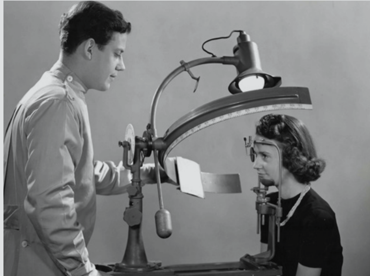
A LASO student measuring the visual field of a patient using an arc perimeter.
